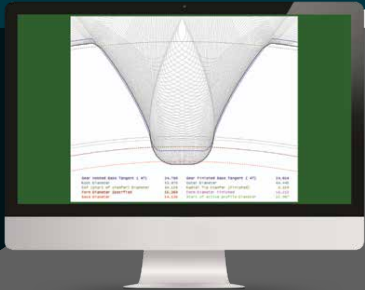
Gear hobbing generated profile to check tool design
