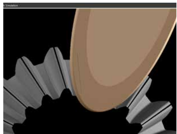
Simulation of dish cutter process in GPS CAM
