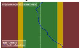
Set ranges for deviation from reference gear surface Pass (green), Fail (red) and Check (yellow)
