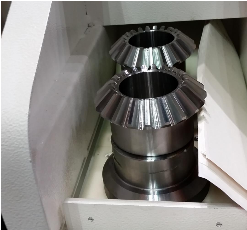
Finished Bevel Gear parts produced during Gear Expo 2015 - 21" tooth bevel with internal spline cut using Standard Sandvik cutters; cycle time 90 minutes from blank.
